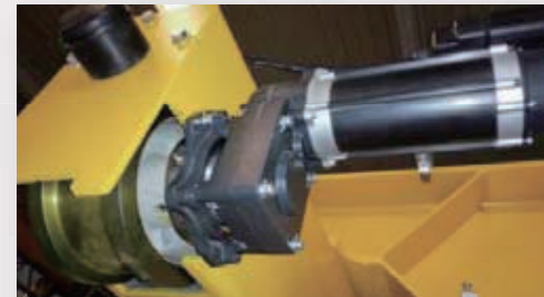
Spline shaft, direct driving
