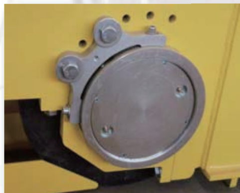
Adjustable vertical inclination and horizontal divergence
